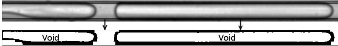
**Figure 8.18:** Determination of  $\varepsilon_{exp}$ . The portion of the channel used for the measurement of  $\varepsilon_{exp}$  is indicated, and the resulting binarized image is shown. The void areas are surrounded by the fluid-fluid and wall-fluid interfaces (in black).
